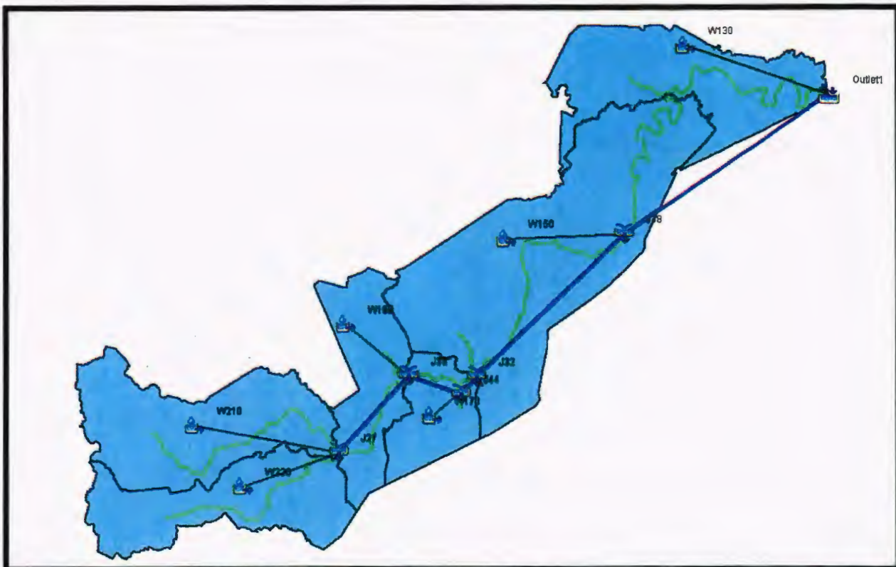
Figure 5-5. HEC-HMS Sub-Basin Boundary and Boundary Condition Lines
